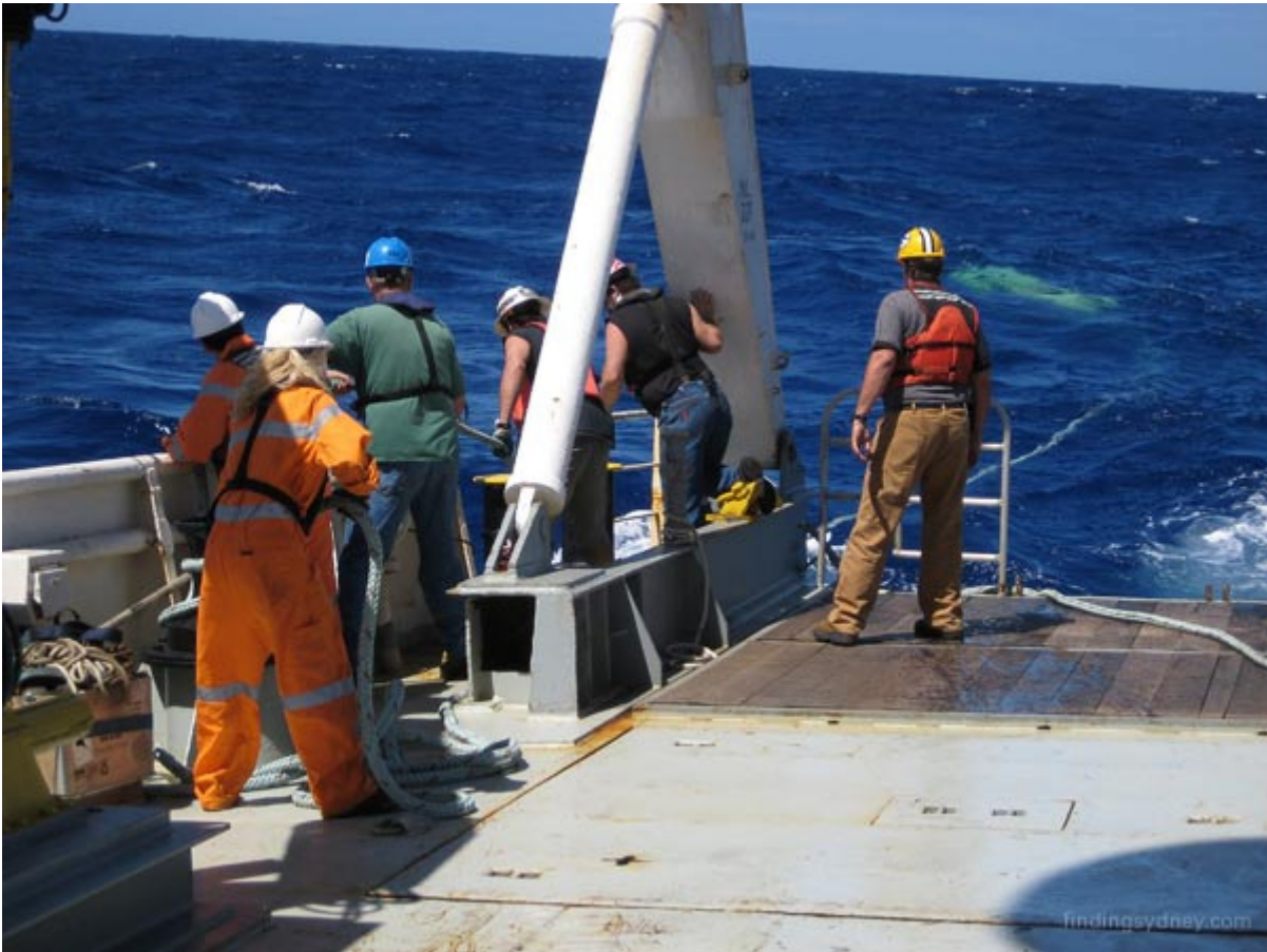
Above Photograph - Hauling the SM30 sonar towfish back towards the vessel.
